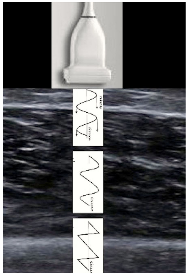
Fig. 20. Tissue non-linearity. A simulated sinusoidal wave from the transducer is continuously distorted at increasing depths due to variation in the speed of sound in soft tissue. In the compressional phase, the propagation speed increases, whereas it decreases during decompression. As the wave propagates, it undergoes progressive distortion from a sinusoidal wave in the near field to a sawtooth pattern at increasing depth. This distorted wave can be represented as a Fourier series containing higher harmonic contributions, the dominant being the second harmonic (twice the transmit or fundamental frequency). The backscattered second harmonic is detected, allowing higher spatial resolution with less attenuation
